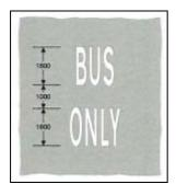
so that the carriageway is marked with the words "Bus Lane" or "Bus Only" with a variation to show that it can be used by cycles.
